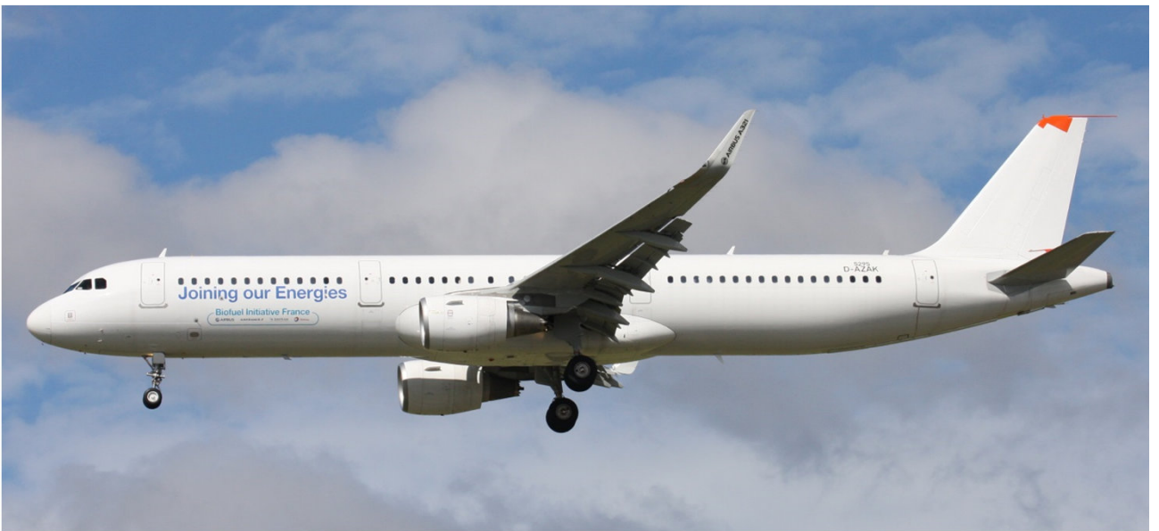
D-AZAK: Special test flight with biofuel by this A321 with sharklets (in cooperation with AIRBUS, AIR FRANCE, SAFRAN and TOTAL).
